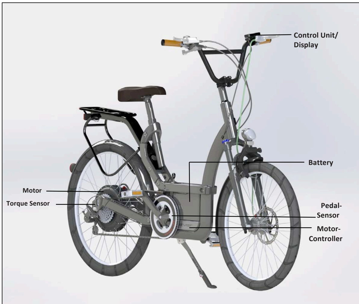
Image 2 complete bike marking: major parts of the electric drive
