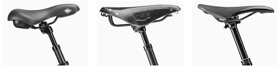
Figure 5. Saddle angle settings for Monday 26 (left), mixed use (middle) and MTB use (right).
