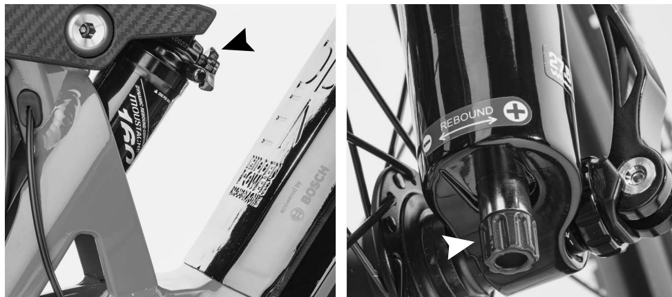
Figure 25. Example of rebound adjustment dials: on the left is for a shock, on the right for a fork.
